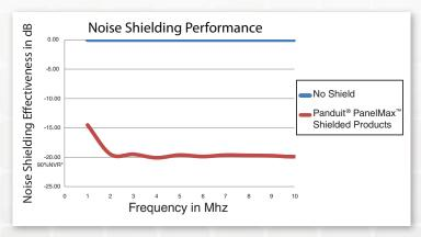
Relative noise reduction in decibels over frequency range of Panduit<sup>®</sup> PanelMax<sup>™</sup> Shielded Wiring Duct and Noise Shield
