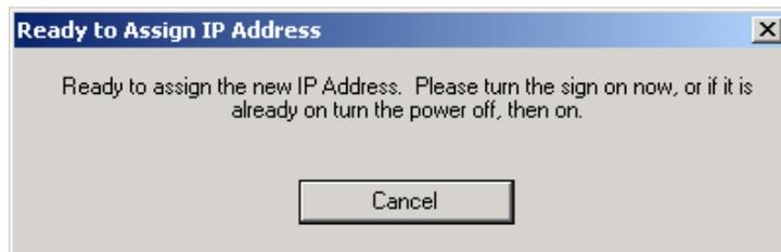
10. You need to either turn the display on or power cycle the display if it is already turned on. Upon successful assignment of an IP Address, the following window appears:
