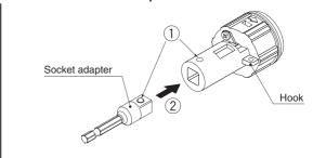
**3.** Connection with tools such as an air driver is also possible. Note) Ensure the TKS does not shake or vibrate.
