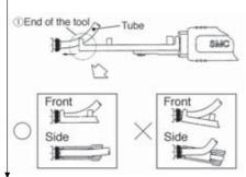
After inserting, grasp the handle tightly and insert the end of the tubing to the stroke end.
