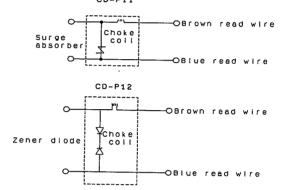
(4) Connection of contact protective box Connect contact protective box with the switch by using lead wire with indication "SWITCH" of the box and lead wire of the switch.
