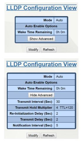
**Mode:** The LLDP mode can be Enabled, Disabled, or Auto. In Auto mode, LLDP is inactive until a switch sends a wake up packet. The default is Auto.
