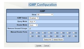
**IGMP Status:** This field indicates whether the IGMP is enabled or disabled. The default value for this field is *Enabled*.
