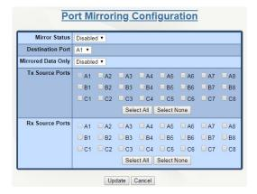
Mirror Status: Enable or Disable the Mirroring functionality by selecting the option in the drop-down menu.
