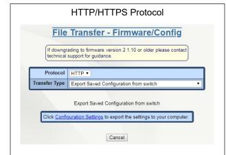
Click on the *Configuration Settings* link to export the settings to your computer. This option allows administrators to back up their configurations to an offsite server in case a custom configuration must be reloaded at a later time.
