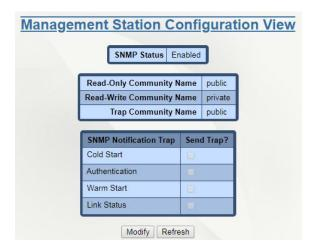
**SNMP Status:** This field indicates whether SNMP is enabled or disabled.
