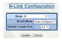
Show: View the ports that are available to install (Modules) currently installed or currently linked up.
