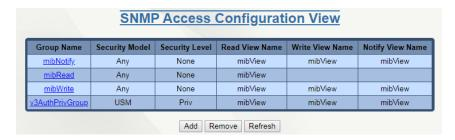
Click on the *Add* button to define new access settings for a group, or click the hyperlink under Group Name to modify existing access for a group. Click the *Remove* button to display a list of current configured group and access settings, with an option to remove specific ones.
