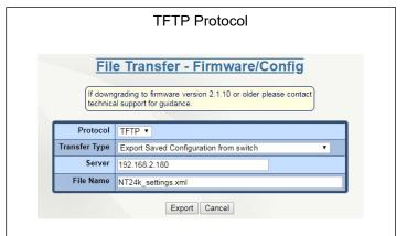
**Server:** This field displays the IP address of the TFTP server.
