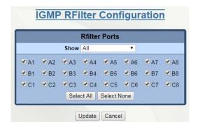
From this dialog window, the administrator selects which ports to identify as RFilter ports and can view all possible ports (Modules), currently installed ports or currently linked up ports. Click on the *Update* button when done with required changes. To save the changes made, return to the Configuration menu and click on the *Save* button.
