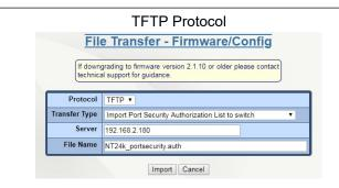
**Server:** This field displays the IP address of the TFTP server.
