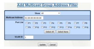
Enter a valid Multicast Group Address and VLAN ID, then select the port(s) to which matching packets will be directed.
