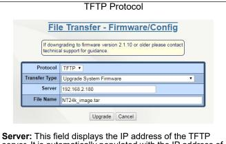
**Server:** This field displays the IP address of the TFTP server. It is automatically populated with the IP address of the PC which is connected to the switch.
