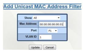
Click on the Update button to add the unicast address and return to the Display Static Unicast MAC Addresses dialog window.
