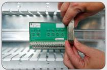
Then routes the cable through the wire duct and snaps the other end of cable to the 1492 IFM Module.
