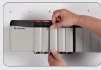
Assembler removes pre-wired 1492 cable from the box and connects the PLC end of the cable to the PLC.
