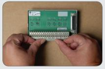
The assembler removes the Bulletin 1492 Interface Module (IFM) from its box and applies the supplied preprinted labels to mark the terminals.
