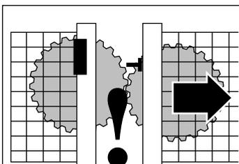
Check the machine is isolated and stopped whenever the interlocked guard door is open.
