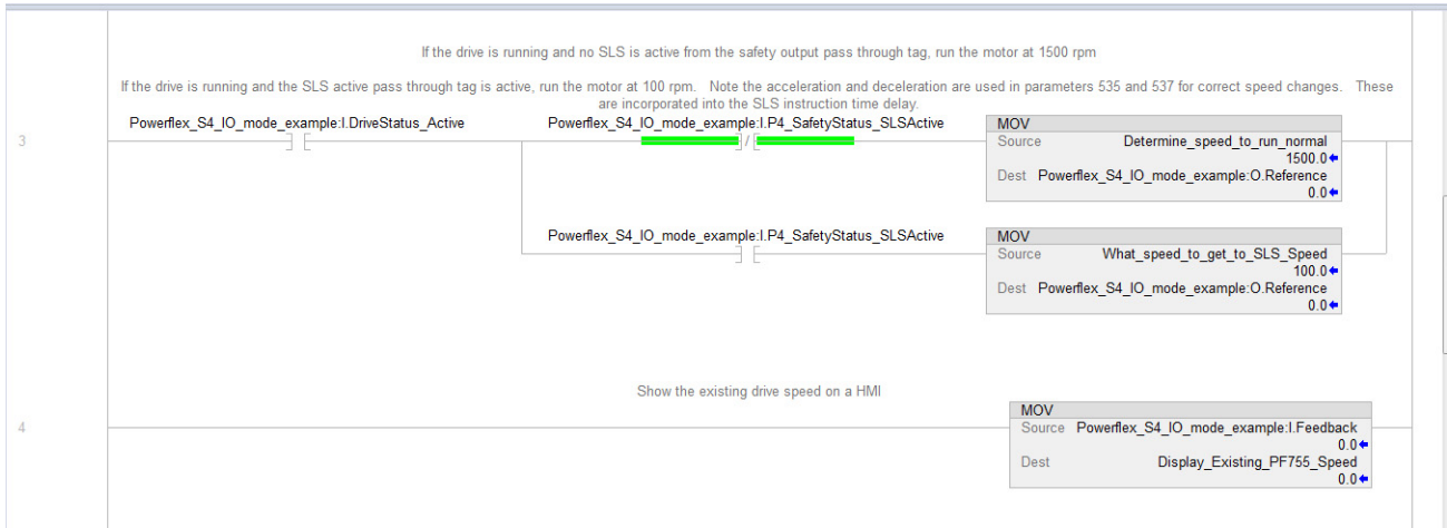
Figure 59 - Standard I/O Routine That Runs the Drive at Velocity and Changes to Safe Limited Speed Velocity When Requested by the Safety Task
