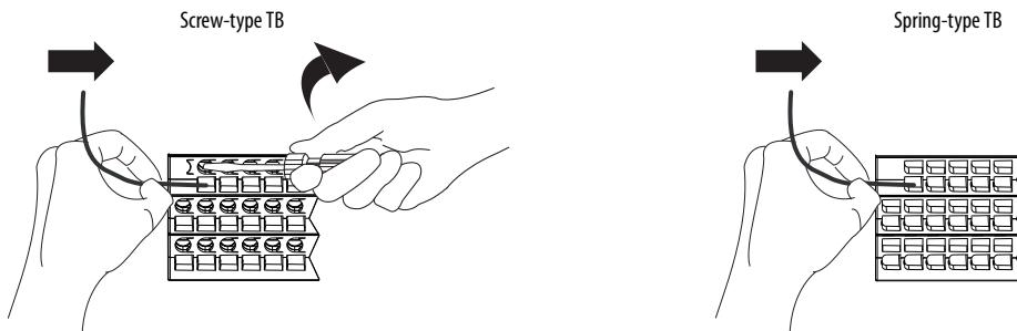
4. Connect individual output relay contact wiring to terminals 1...46 as indicated in [Wiring Connections for 5094-OW4IS and 5094-OW4ISXT on page 11](#). The even-numbered terminals are one pole of the relay contacts; the odd-numbered terminals are the other pole of the relay contacts.
