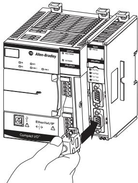
3. Tighten the screws on both sides of the serial cable.
