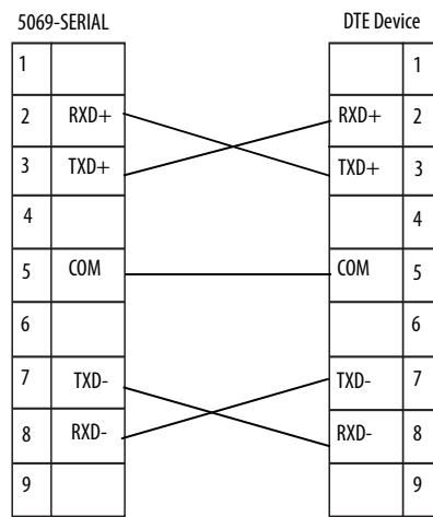
**RS-485****5069-SERIAL RS-485 Wiring**
