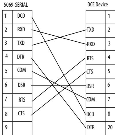
**5069-SERIAL to DTE Device with "Full or Half-duplex" or Null Modem**
