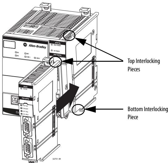
7. Verify that the module is installed in one of the following ways:
