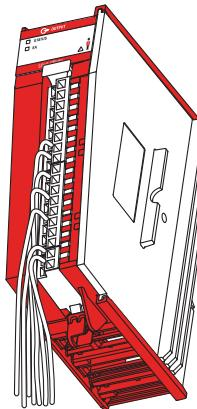
3. Thread the cable tie through the lower hook at the bottom of the RTB.
