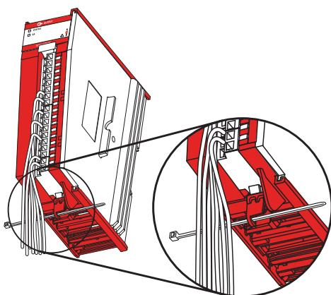
5. Wrap the cable tie around the wires and secure it.
