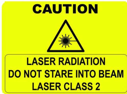
Figure 83 - 450L-E Laser Warning Label (Positioned on the Backside of the Aluminum Profile)
