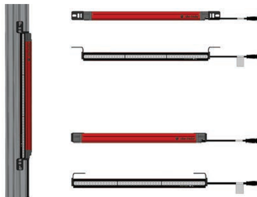
Figure 52 - 450L Safety Light Curtain Mounted Backwards on an Extruded Aluminum Profile Using the Standard Top/Bottom Mounting Bracket
