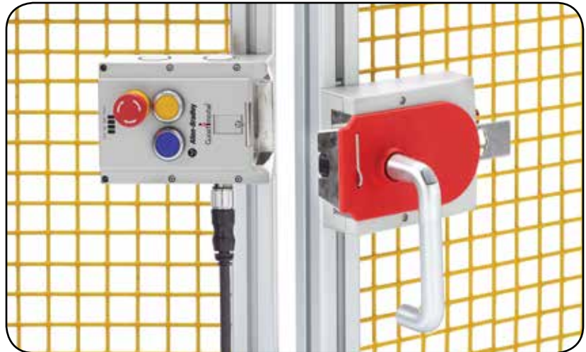
Right-hand Multifunctional Access Box mounted on a hinged guard.
