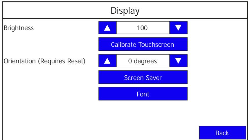
Follow these steps to complete the calibrate touch screen procedure. This process must be done by physically touching the screen. Use a plastic stylus device with a minimum tip radius of 1 mm (0.040 in.) to prevent damage to the touch screen.
