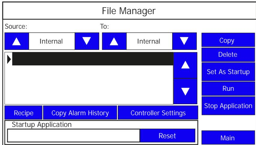
**IMPORTANT** The Stop Application button is only available in firmware revision 3.011 onwards.
