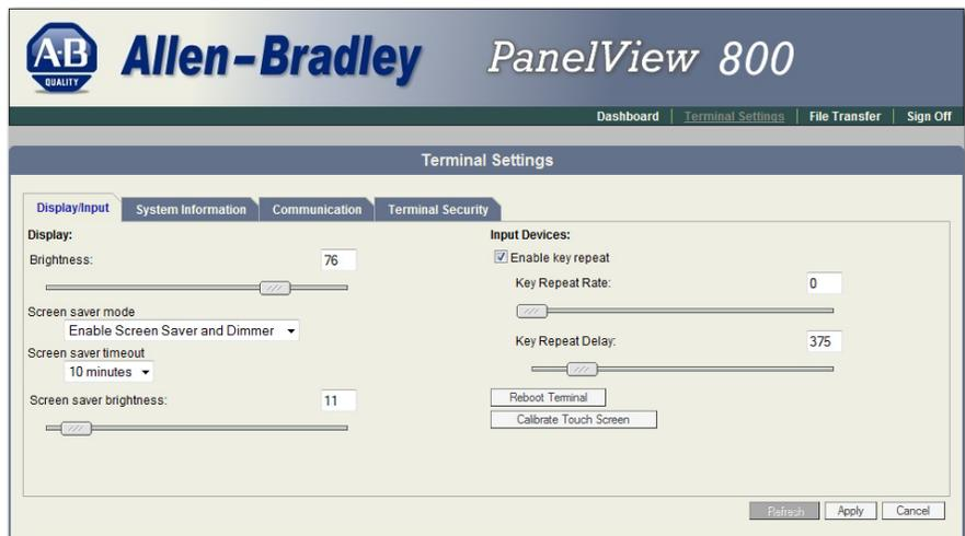
5. Drag the slider under Key Repeat Rate to adjust the speed at which a character repeats when a key is held down.
