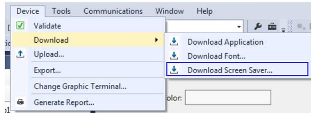
2. Browse your computer for the screen saver, then select it and click Open. The Connected Components Workbench software connects to the terminal and downloads the screen saver.
