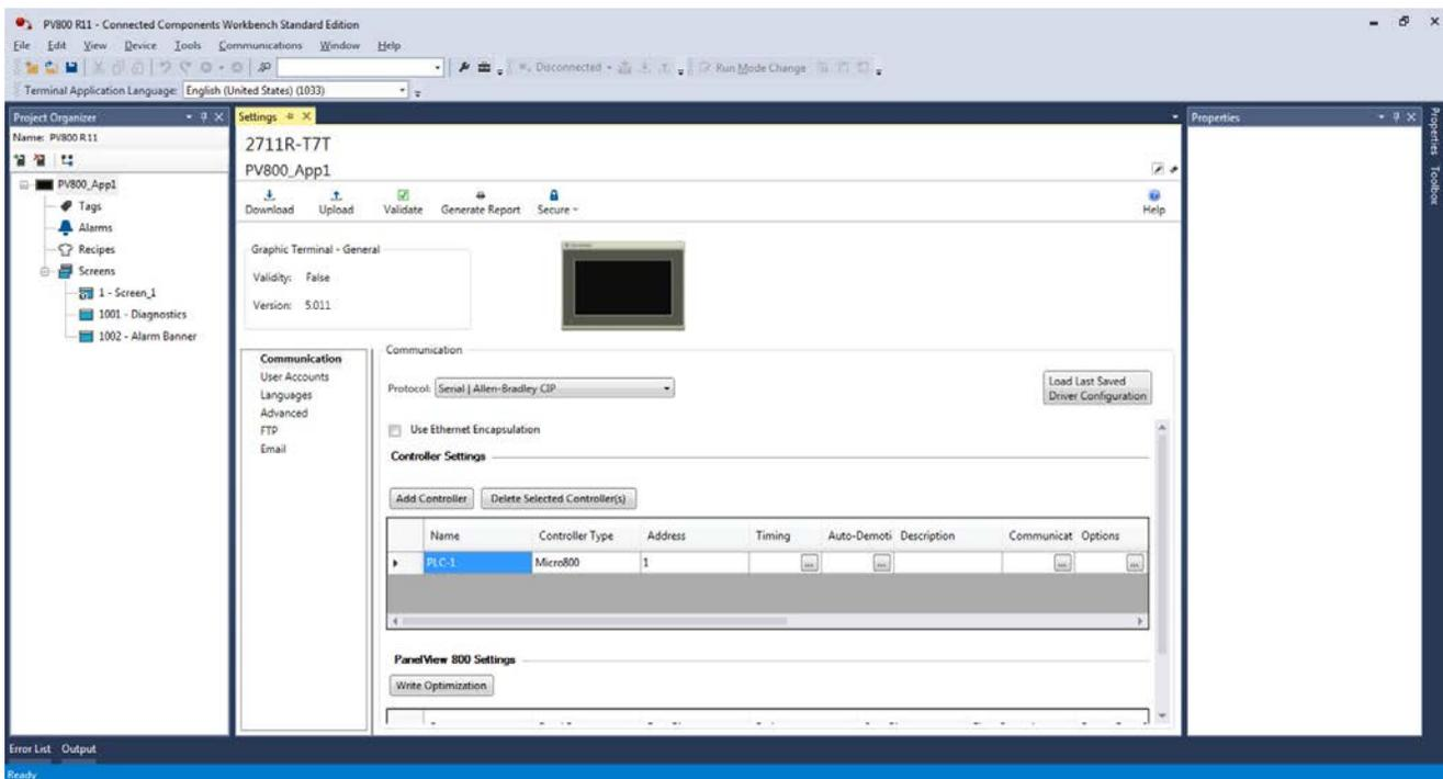
We strongly recommend that you validate the transferred application using the terminal software before running the application. Non-validated applications, when started on the terminal, display a reminder pop-up message that the application is not validated. Applications designed for the CompactLogix 5370 controllers must be validated before running on the terminal.
