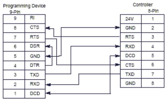
The maximum cable length for serial communication is 15.24 m (50 ft) at 19.2 Kbps
