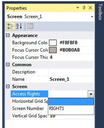
**IMPORTANT** You cannot secure a screen unless rights are defined and assigned to users on the User Accounts screen in the Settings tab.
