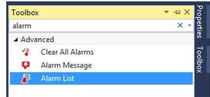
3. Right-click the Alarm List object and select Properties. Configure the properties as required.
