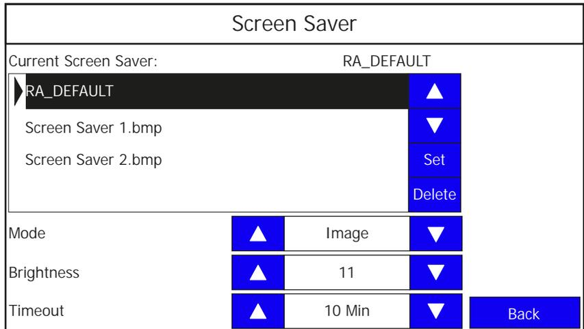
4. Use the up and down arrow keys to select the screen saver, then press Set to use it or Delete to remove it from the terminal.
