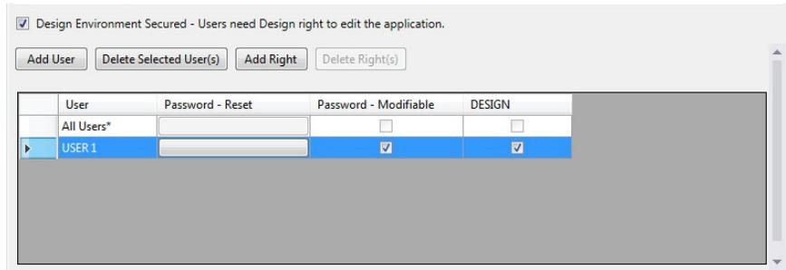
To reset a password for any user, click the Password - Reset cell and the Security - Reset Password dialog appears. You can enter a new password without knowing the old password.
