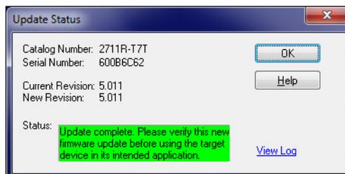
11. Open the system information screen on the terminal to verify that the new firmware version is correct.
