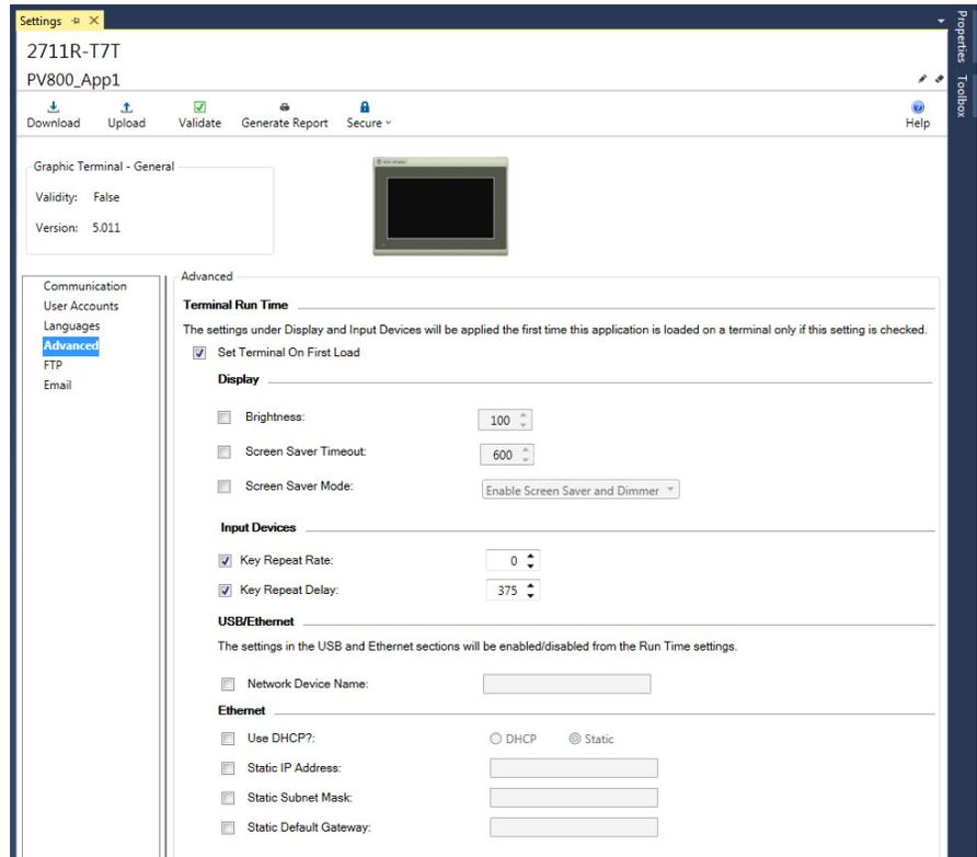
4. Under Input Devices, select the checkbox for the setting you want to configure.
