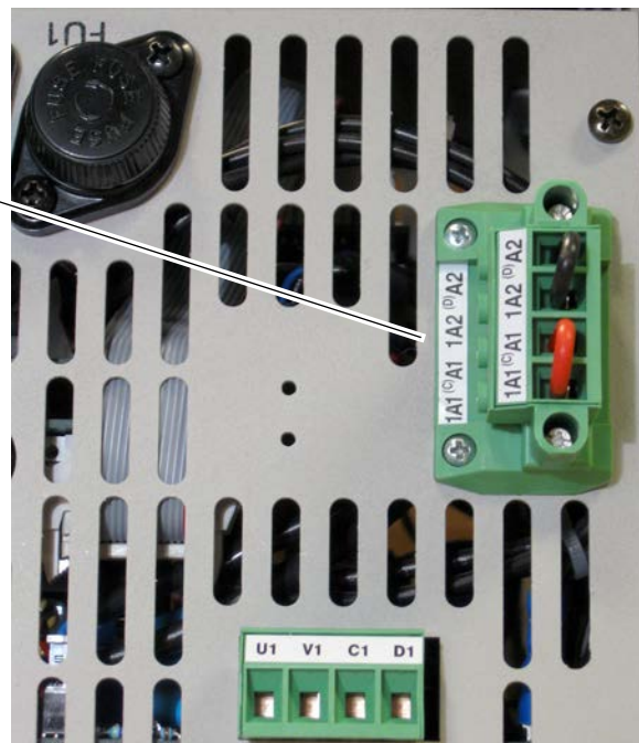
Figure 28 - Frame B Armature Voltage Feedback Circuit Terminal Block Location
