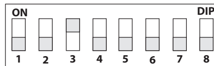
Figure 57 - Drive Size DIP Switch S15 Example
