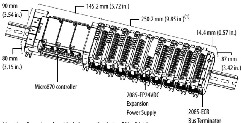
Mounting dimensions do not include mounting feet or DIN rail latches.
