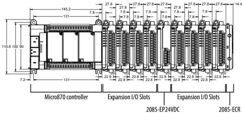
Measurements in millimeters
