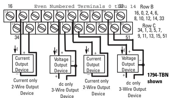
**Wiring Connections for the 1794-IE4XOE2XT/B 4 Analog Input/2 Output Module**
