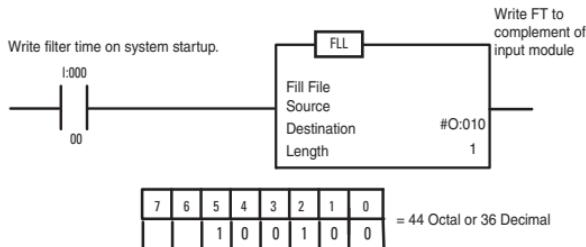
To increase the filter time, set the bits according to the table below.
