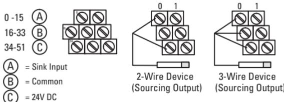
**IMPORTANT** To comply with the CE Low Voltage Directive (LVD), all connected I/O must be powered from a source compliant with the following: Safety Extra Low Voltage (SELV) or Protected Extra Low Voltage (PELV).
