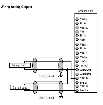
Analog outputs may fluctuate for less than a second when power is applied or removed. This characteristic is common to most analog outputs. While the majority of loads will not recognize this short signal, take preventative measures to make sure that connected equipment is not affected. Failure to take these preventative measures may result in unexpected load reactions.
