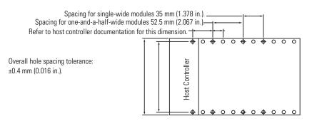
Panel Mounting By Using the Modules as a Template
