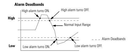
The module checks for an alarm deadband value that is less than 0 or large enough to be equal to or exceed one-half of the difference between the high alarm and low alarm values. When one of these conditions occurs, a module configuration fault results.
