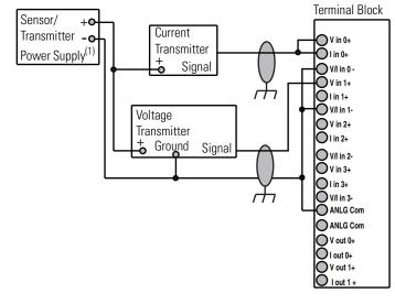
(1) The sensor power supply must be rated Class 2.
