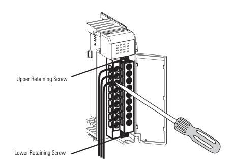
When wiring the terminal block, keep the finger-safe cover in place.
