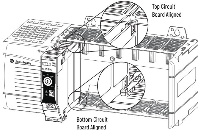
2. Slide the module into the chassis until it snaps into place.
