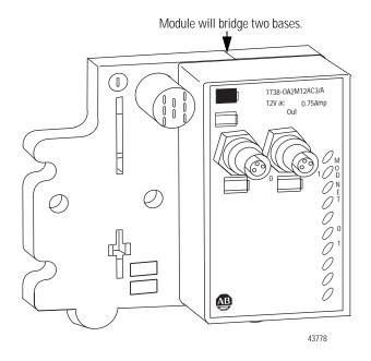
**3.** Push the module down until it engages the latching mechanism. You will hear a clicking sound when the module is properly engaged.
