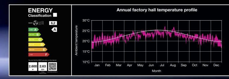
Rittal specifies the SEER to indicate the actual efficiency of a cooling unit, since a precise calculation must also consider the seasonal temperature variation. The standard point for determining the EER does not make allowance for actual fluctuations in hall temperatures.
