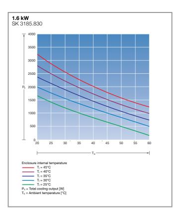
Output class 2000/2600 W (110 - 240 V, 1 ~, 50 - 60 Hz / 380 - 480 V, 3 ~, 50 - 60 Hz)
