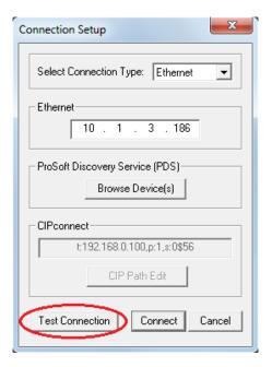
**5** If the *Test Connection* is successful, click **CONNECT**. The *Diagnostics* window is now accessible.
