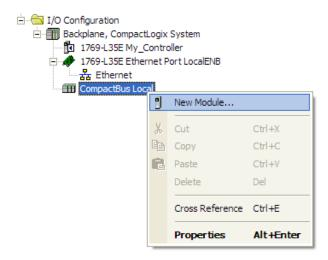
This action opens the *Select Module Type* dialog box. In the *Module Type Vendor Filters* area, uncheck all boxes except the **ProSoft Technology** box. A list of ProSoft Technology modules will appear below.
