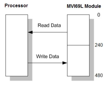
Database address 0 to 239 is continuously transferred from the module to the processor. Database address 240 to 479 is continuously transferred from the processor to the module.
