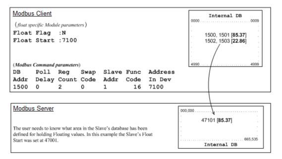
**Float Flag: "N"** tells the Client to ignore the floating values and treat each register data as a data point composed of 1 word, 2 bytes or 16 bits.
