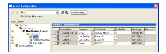
6 If the module is not located in the default slot (or is in a remote rack), edit the connection input and output variables that define the path to the module in the **FINAL NAME** column (**NAME** column for RSLogix version 16 or less). For example, if your module is located in slot 3, change *Local:1:I* in the **FINAL NAME** column to *Local:3:I*. Do the same for *Local:1:O*.
