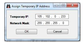
**Important:** The temporary IP address is only valid until the next time the module is initialized. For information on how to set the module's permanent IP address, see page 58.
