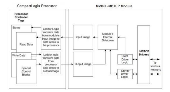
All data transferred between the module and the processor over the backplane is through the input and output images. Ladder logic is needed in the CompactLogix processor to interface the input and output image data with data defined in the Controller Tags. All data used by the module is stored in its internal database. This database is defined as virtual MBTCP data tables with addresses from 0 to 239 each.
