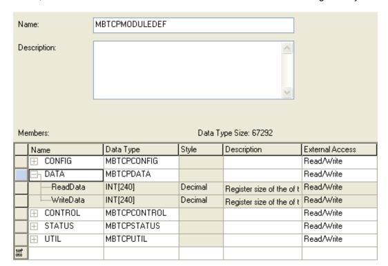
Notice that these UDTs are the data types used to declare the MBTCP.DATA.ReadData and MBTCP.DATA.WriteData controller tag arrays. The UDTs are commented in the Description column.
