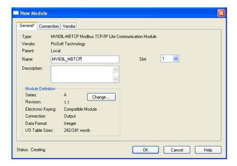
The MVI69L-MBTCP module will now be visible at the I/O Configuration tree.
