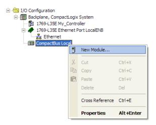
This action opens the *Select Module Type* dialog box. Enter **generic** in the search text box and select the **GENERIC 1769 Module**. If you're using an earlier version of RSLogix, expand **OTHER** in the *Select Module* dialog box, and then select the **GENERIC 1769 MODULE**.
