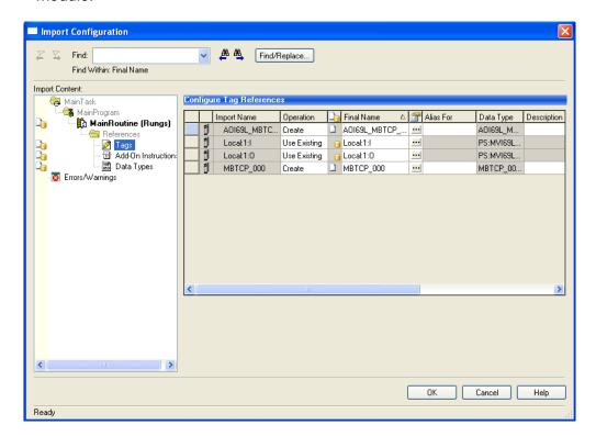
9 Associate the I/O connection variables to the correct module in the corresponding slot number. The default values are Local:1:I and Local:1:O. You must edit these values if the card is placed in a slot location other than slot 1 (Local:1:x means the card is located in slot 1). Since the second card is placed in slot 2, change the *Final Name* to Local:2:I and Local:2:O. Also, you can append a '\_2' at the end of the *Final Name* of 'AOI69\_MBTCP' and 'MBTCP' arrays as shown below.
