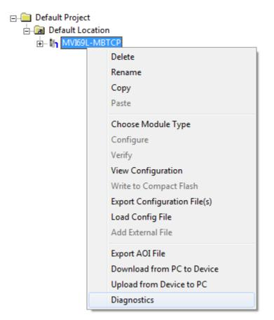
**3** After the *Diagnostics* window opens, click the **SETUP CONNECTION** button to browse for the module's IP address.
