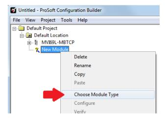
3 Select the MVI69L-MBTCP module to add a second (or more) module in the PCB project.
