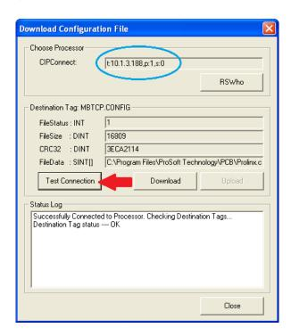
5 When ready, click DOWNLOAD to download the configuration file to the processor. Following the download process, the module will automatically be rebooted.
