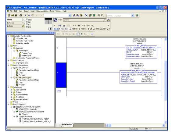
The setup procedure is now complete. Save the project, it is ready to download to the CompactLogix processor.
