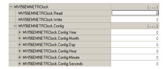
The bit will be automatically reset and the current clock value will be copied to **MVI56MNETRCLOCK.CONFIG** controller tag as follows.
