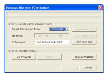
2 Configure the path as shown in the following illustration, and click CONSTRUCT CIP PATH to build the path in text format.
