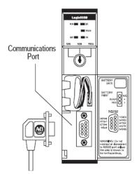
**2** Connect the straight connector end of the cable to the serial port on your computer.
