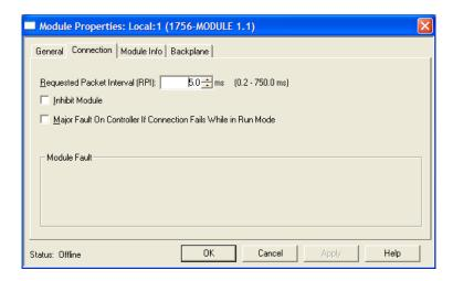
3 Save the module. Click **OK** to dismiss the dialog box. The **CONTROLLER ORGANIZATION** window now displays the module's presence.
