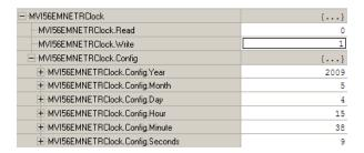
The bit will be automatically reset to 0.
