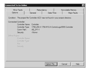
5 In the *Connected To Go Online* dialog box, click the **GENERAL** tab. This tab shows information about the processor, including the Revision (firmware) version. In the following illustration, the firmware version is 11.32
