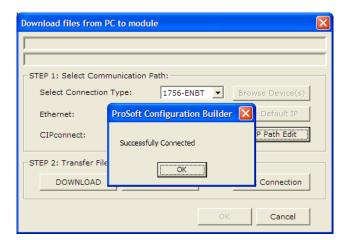
5 Click **OK** to close the Test Connection pop-up and then click **DOWNLOAD** to download the configuration files to the module through the path.
