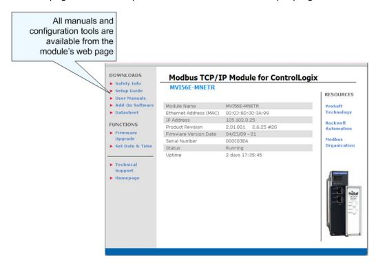
**Important:** The temporary IP address is only valid until the next time the module is initialized. Please refer to Setting Temporary IP Address (page 19) in the MVI56E-MNETR User Manual for information on how to set the module's permanent IP address.
