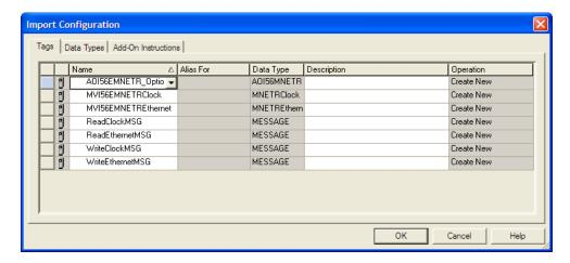
The Add-On Instruction will be now visible in the ladder logic. Observe that the procedure has also imported data types and controller tags associated to the Add-On Instruction.
