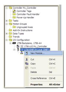
6 Repeat steps 2 and 3 to add the second EtherNet/IP module to the remote rack.
