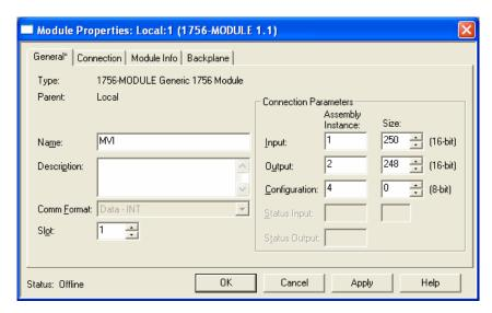
3 In the **SLOT** field, use the up and down arrows on the right side of the field to select the slot number where the module will reside in the rack, and then click **OK.**
