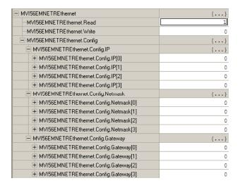
The bit will be automatically reset and the current Ethernet settings will be copied to **MVI56MNETRETHERNET** controller tag as follows.
