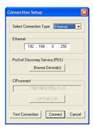
3 If *PCB* is still unable to connect to the module, click the **Browse Device(s)** button to open the *ProSoft Discovery Service*.
