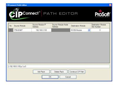
The CIPconnect Path Editor allows you to define the path between the PC and the MVI56E-MNETR module. The first connection from the PC is always a 1756-ENBT (Ethernet/IP) module.
