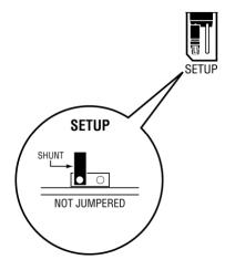
**Note:** If you are installing the module in a remote rack, you may prefer to leave the Setup pins jumpered. That way, you can update the module's firmware without requiring physical access to the module.
