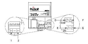
**Attention:** When connecting wiring, torque terminal screws to 7 to 9 inch-pounds.
