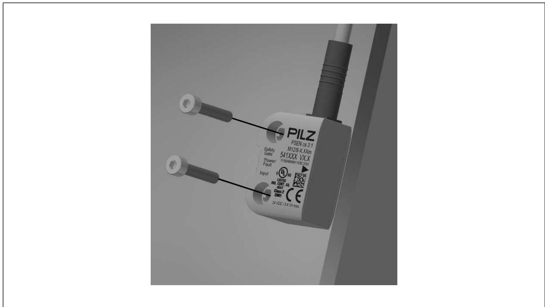
3. Attach the screws for the actuator, leaving a distance of 3 ... 6 mm between the screw head and plate.
