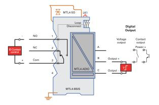
The MTL4-BSISR, for IS field devices or MTL4-BSGPR, for non-IS field devices, is used with the MTL4-ADIO isolator for digital output applications where a relay contact is required. Normally open (NO) and normally closed (NC) contacts are provided Inductive loads must be suppressed.
