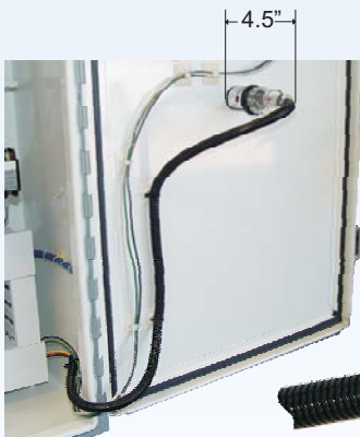
Part#: R-3W-DR-C6 Door mount kit for additional voltage protection. Includes a 30mm adapter and 6' of NW10 flexible conduit. (With bending radius, allow for 4.5" depth into panel)
