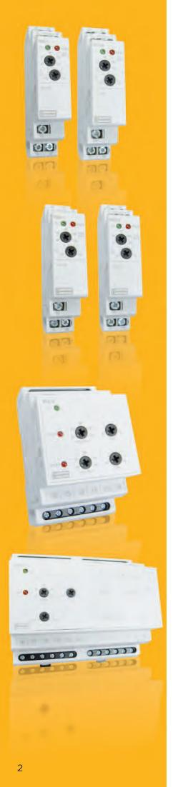
AC current protectors provide a continuous surveillance of monitored circuits and offer user adjustable trip points (set points) with time delay settings. When the current moves outside the set point limit for longer than the time delay, the relay will operate providing an alarm control or tripping signal.
