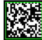
Quiet zone violation
