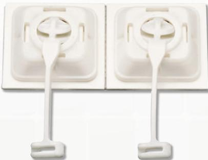
The opening and closing motion of an enclosure door is a common cause of failure of control systems that feature control lights, touch pads, and switches in the panel door. The Panduit dynamic cable manager provides a reliable and cost-effective method for ball-and-socket tether design securing cable bundles that pass across the enclosure door hinge. The ball-in-socket design of the mount prevents excessive strain on the wiring and the mount, improving the overall system reliability.
