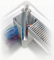
Panduct® PanelMax™ Corner Wiring Duct is an innovative one-piece wire management product that makes more efficient use of space inside enclosures, speeds installation, and reduces control panel assembly costs. PanelMax™ Corner Wiring Duct is used in the vertical corners of medium to large electrical control panels (with both side and back panels) to route, conceal, and protect electrical wiring.
