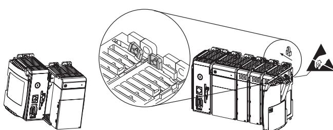
The modules mechanically lock together with a tongue-and-groove design and have an integrated communication bus that is connected from module to module by a moveable bus connector.
